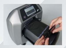
Feed in the imaging plate - intake then starts automatically.
